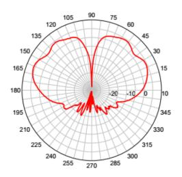
Cable #1 & #2 MGW 5500 MHz – Azimuth Plot
