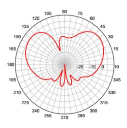
Cable #1 & #2 MGW 5500 MHz – Elevation Plot
