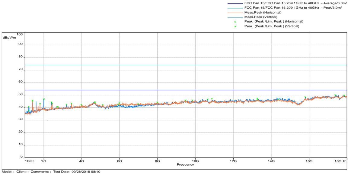
**Test Results: 15.209 Radiated Spurious Emissions Low Channel, Tx at 802.11a 5200MHz**
