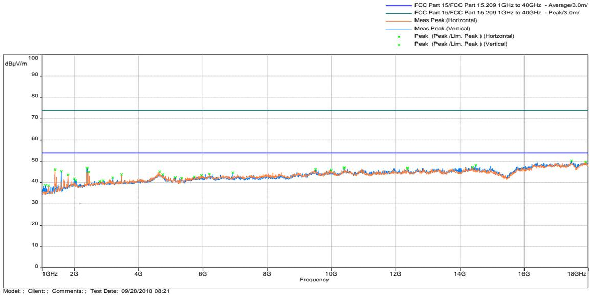
**Test Results: 15.209 Radiated Spurious Emissions Low Channel, Tx at 802.11a 5240MHz**
