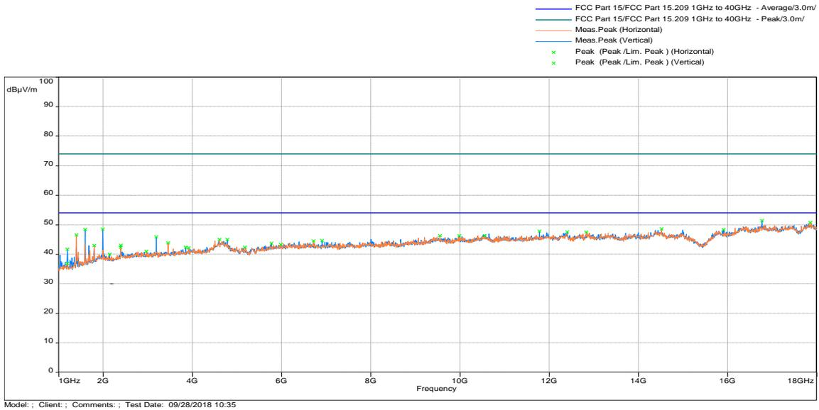
**Test Results: 15.209 Radiated Spurious Emissions Low Channel, Tx at 802.11n 20MHz 5200MHz**
