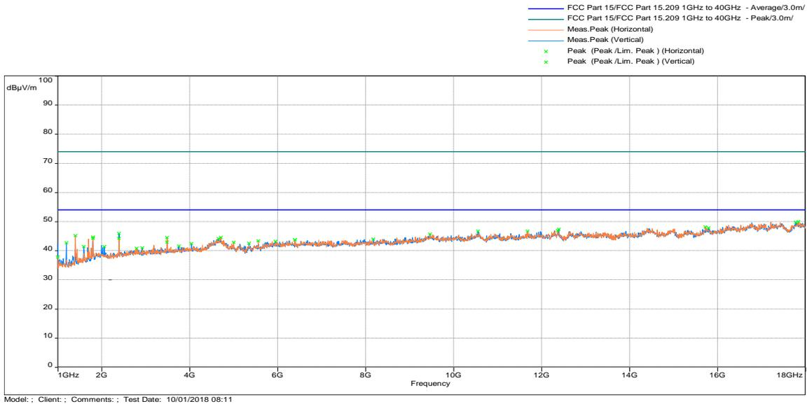
**Test Results: 15.209 Radiated Spurious Emissions Low Channel, Tx at 802.11ac 80MHz 5210MHz**
