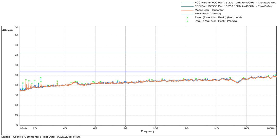
**Test Results: 15.209 Radiated Spurious Emissions Low Channel, Tx at 802.11n 40MHz 5190MHz**
