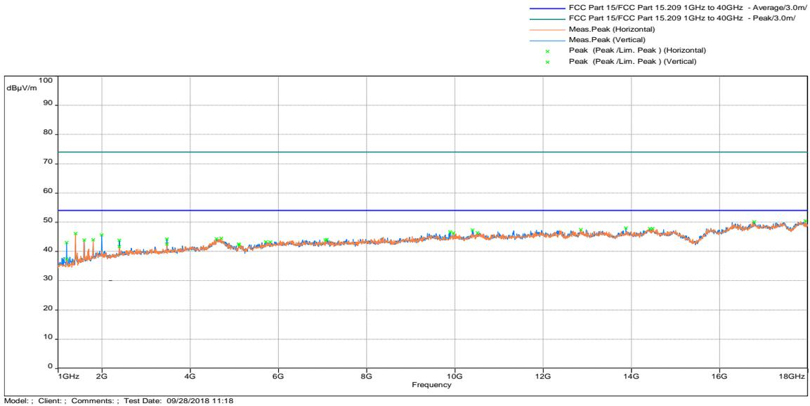
**Test Results: 15.209 Radiated Spurious Emissions Low Channel, Tx at 802.11n 20MHz 5240MHz**
