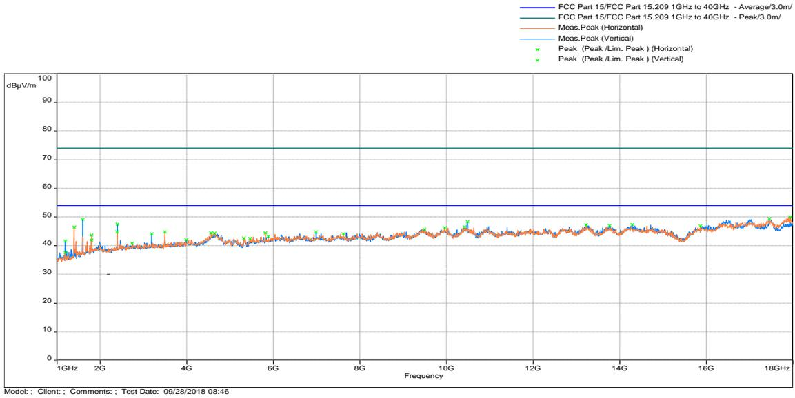
**Test Results: 15.209 Radiated Spurious Emissions Low Channel, Tx at 802.11n 20MHz 5180MHz**
