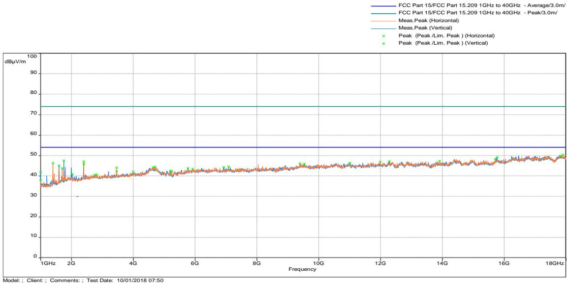
**Test Results: 15.209 Radiated Spurious Emissions Low Channel, Tx at 802.11n 40MHz 5230MHz**
