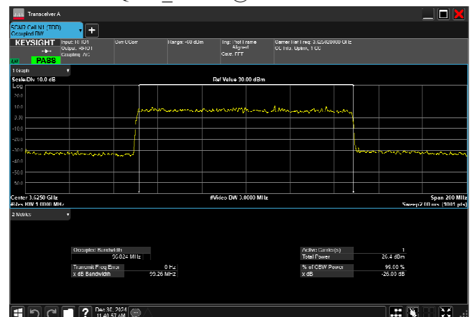
n77_2_100MHz_30kHz_3625MHz_DFT-s-OFDM 256 QAM_RB270@0 96.824MHz
