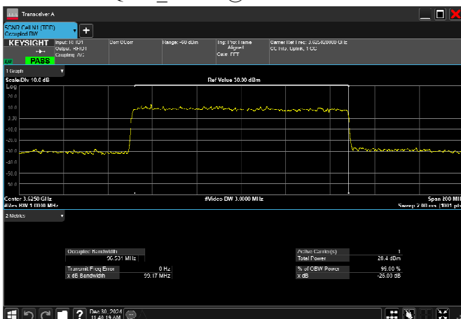
n77_2_100MHz_30kHz_3625MHz_DFT-s-OFDM 64 QAM_RB270@0 96.531MHz
