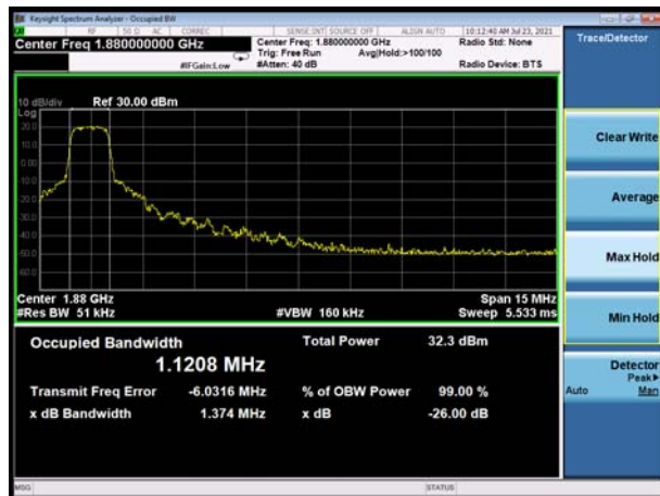
LTE Band 2 15MHz QPSK CH-Middle
