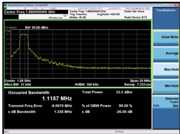
LTE Band 2 20MHz QPSK CH-Middle
