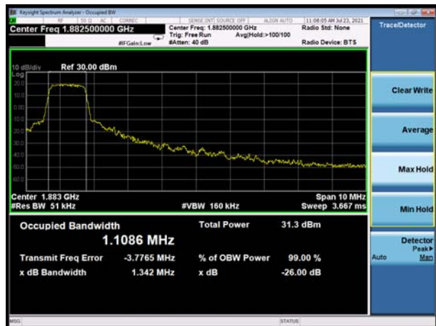
LTE Band 25 20MHz QPSK CH-Middle
