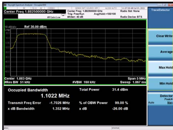
LTE Band 25 15MHz QPSK CH-Middle
