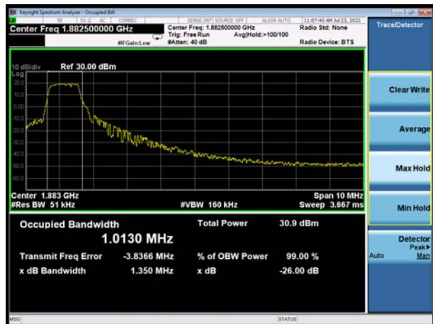
LTE Band 25 20MHz 16QAM CH-Middle
