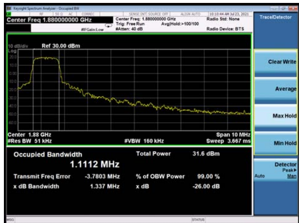
LTE Band 2 20MHz QPSK CH-Middle
