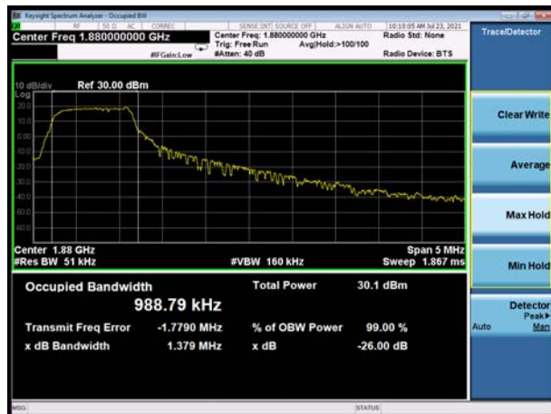
LTE Band 2 15MHz 16QAM CH-Middle
