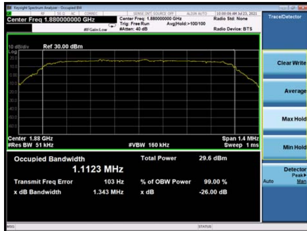
LTE Band 2 5MHz QPSK CH-Middle
