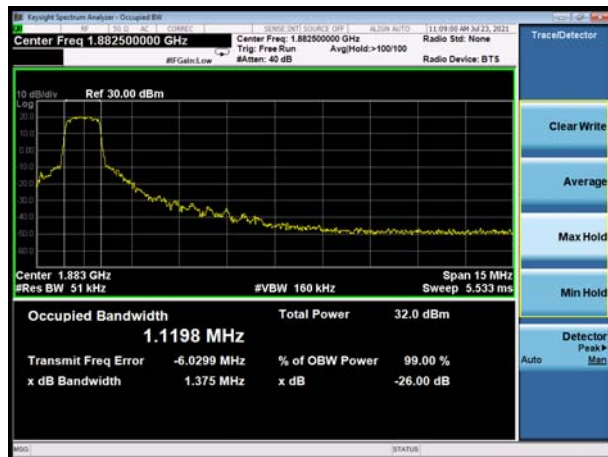
LTE Band 25 15MHz QPSK CH-Middle
