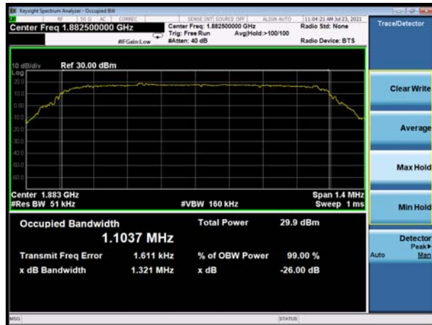
LTE Band 25 5MHz QPSK CH-Middle
