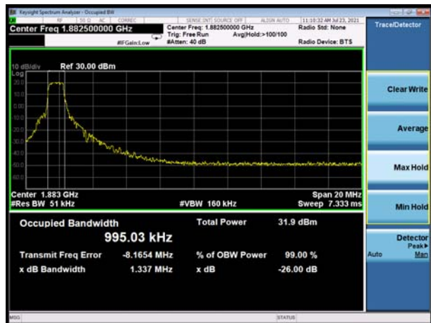
LTE Band 25 20MHz 16QAM CH-Middle
