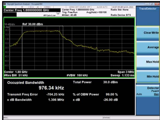
LTE Band 2 10MHz 16QAM CH-Middle
