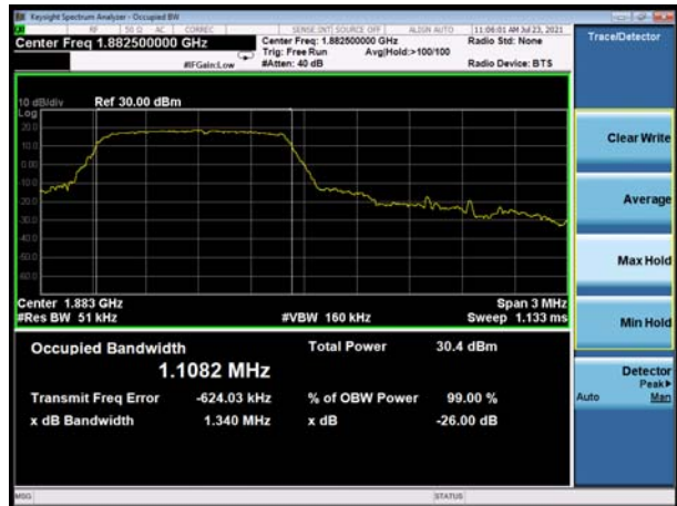
LTE Band 25 10MHz QPSK CH-Middle
