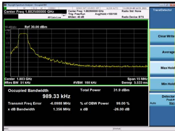
LTE Band 25 15MHz 16QAM CH-Middle
