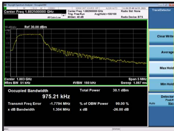
LTE Band 25 15MHz 16QAM CH-Middle
