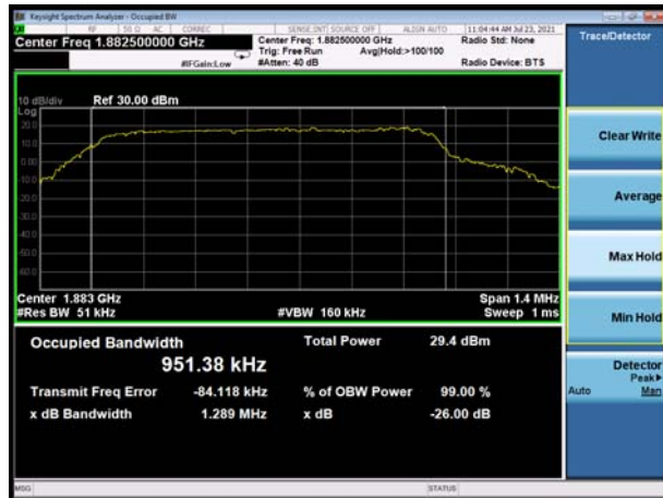
LTE Band 25 5MHz 16QAM CH-Middle
