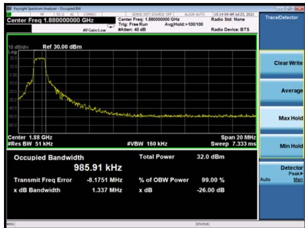
LTE Band 2 20MHz 16QAM CH-Middle
