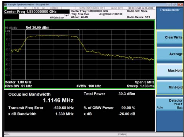
LTE Band 2 10MHz QPSK CH-Middle
