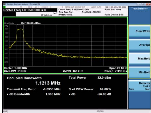
LTE Band 25 20MHz QPSK CH-Middle
