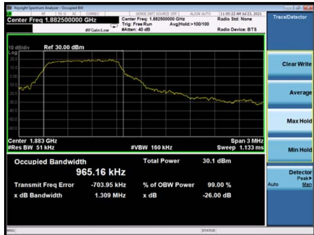
LTE Band 25 10MHz 16QAM CH-Middle
