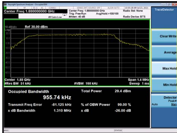
LTE Band 2 5MHz 16QAM CH-Middle
