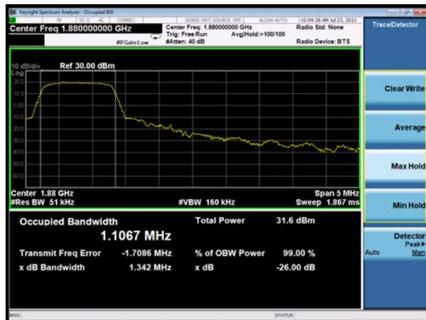
LTE Band 2 15MHz QPSK CH-Middle
