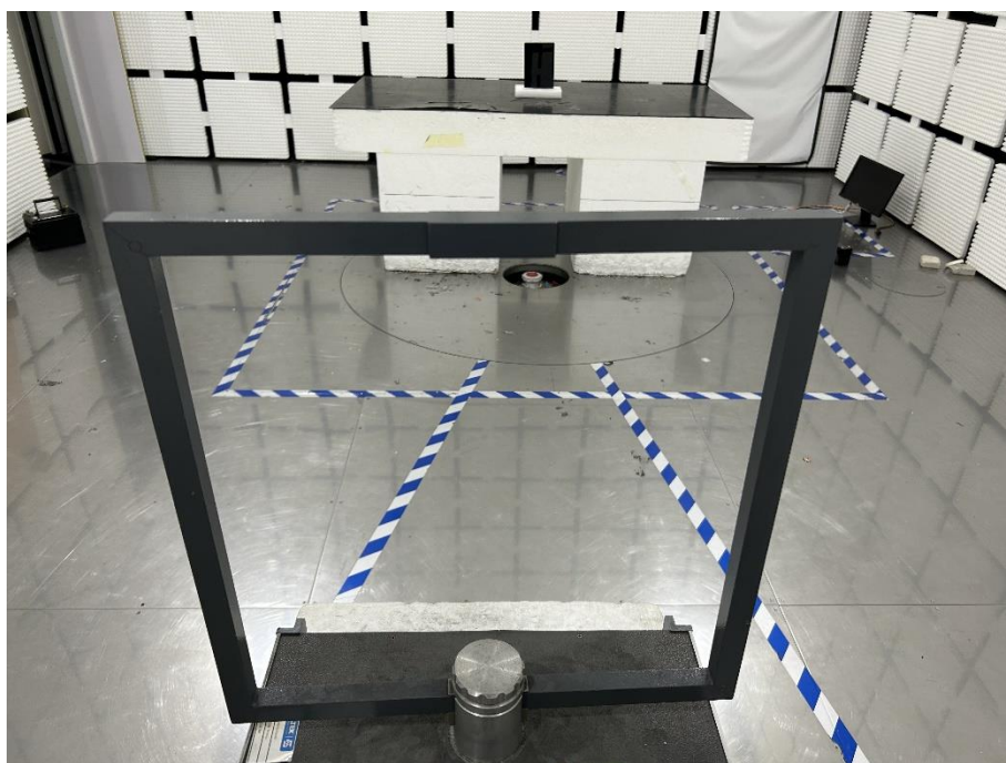
Radiation Emission Test Setup (Below 30MHz)
