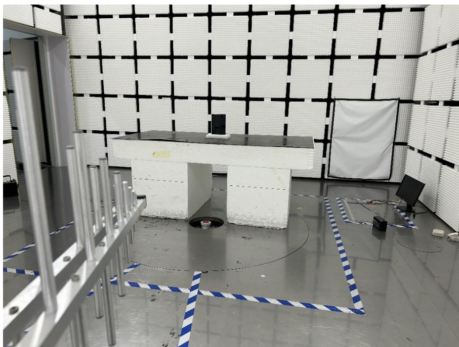
Radiation Emission Test Setup (30MHz to1GHz)
