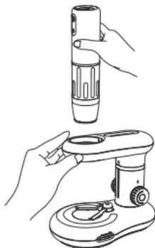
2. Hold the base with one hand and insert the microscope vertically into the installation hole.
