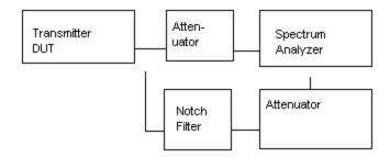
Method of Measuring Conducted Spurious Emissions
