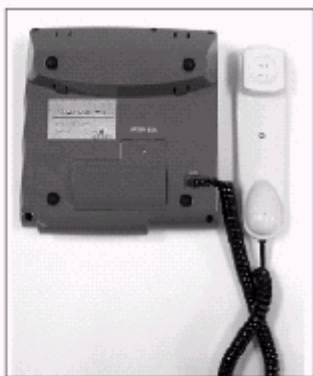
② Insert the battery & connector
