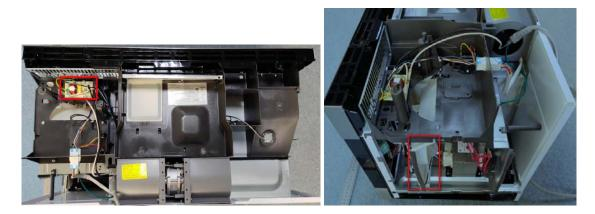
The new position of fuse PCB board and fan has changed.
