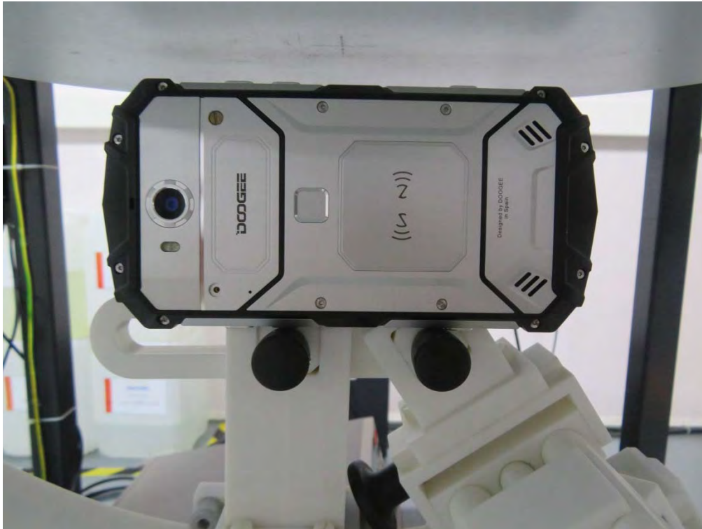
10mm body-worn Left Side Setup Photo (hotspot)
