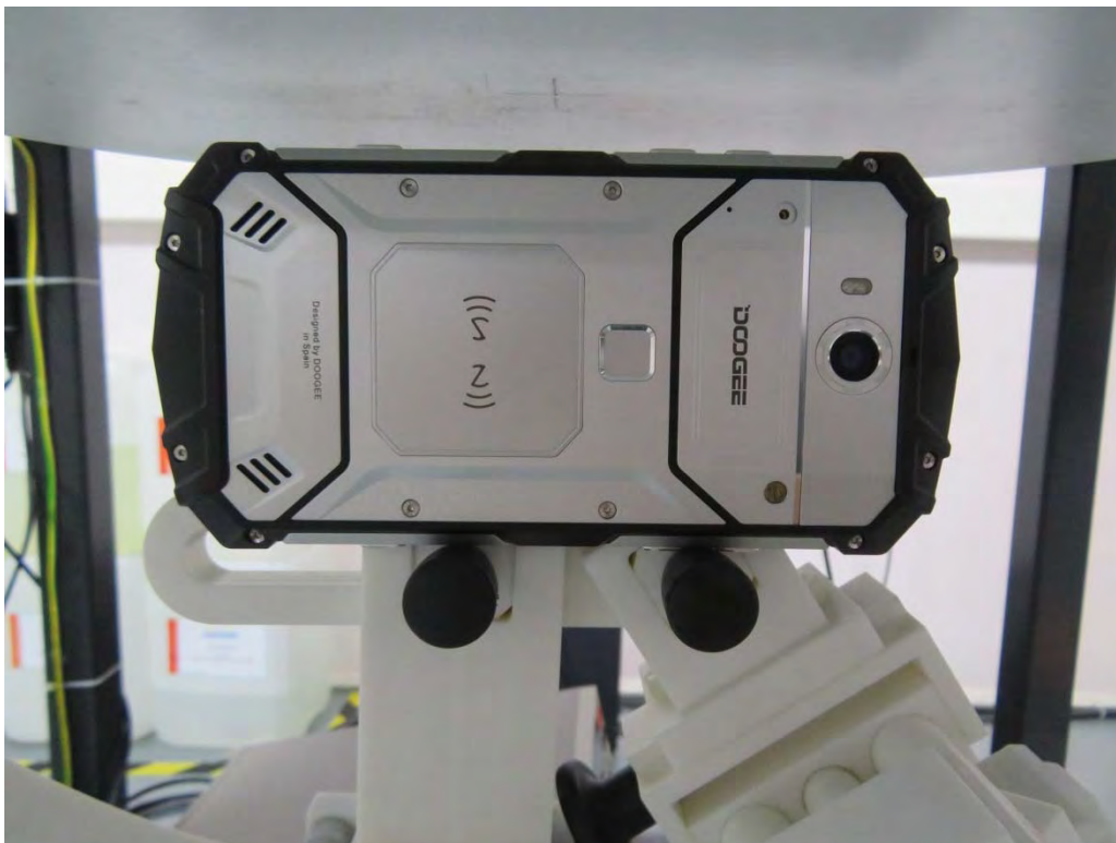
10mm body-worn Right Side Setup Photo (hotspot)
