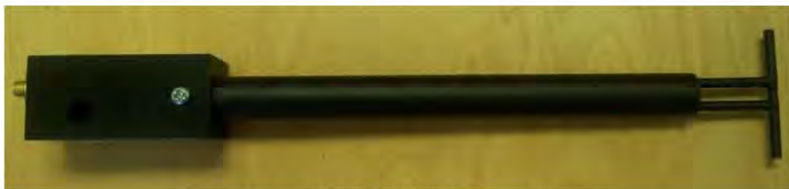
Figure 1 – MVG COMOSAR Validation Dipole
