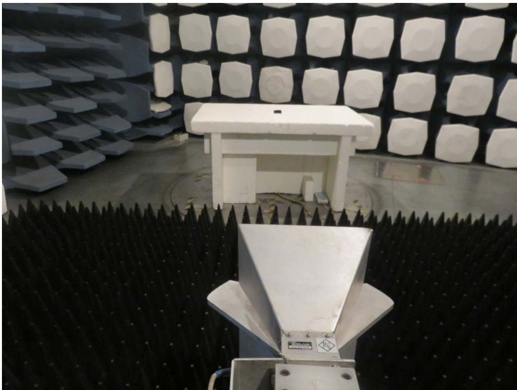
Picture 1: Radiated Spurious Emissions Test setup
