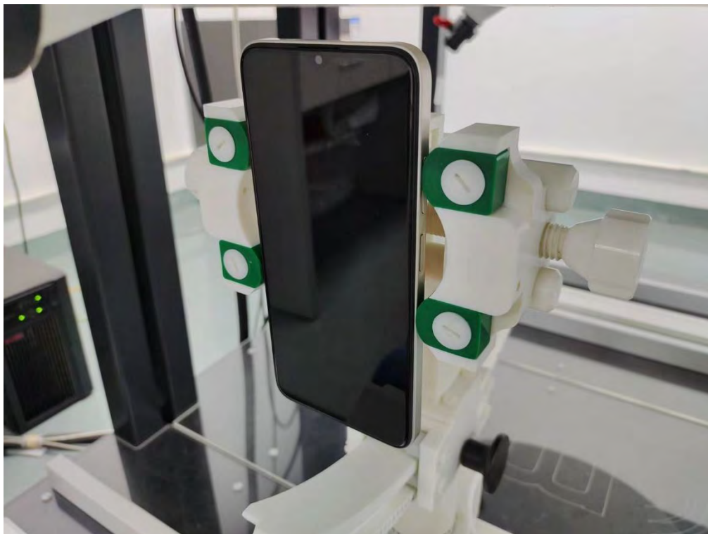
Body Top side (separation distance is 10mm)
