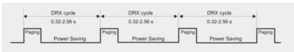
Figure 31: Power saving and paging in LTE networks
