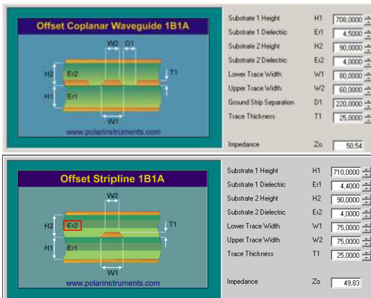
Figure 14: Embedded Stripline line arrangement
