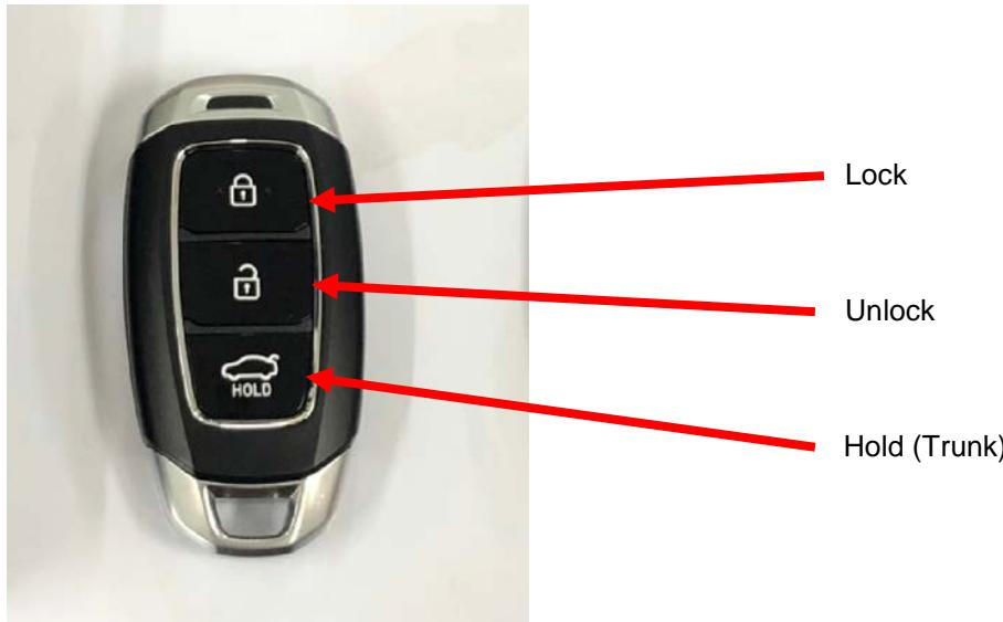
You can lock, unlock, trunk and hold your vehicle with this remote transmitter.
