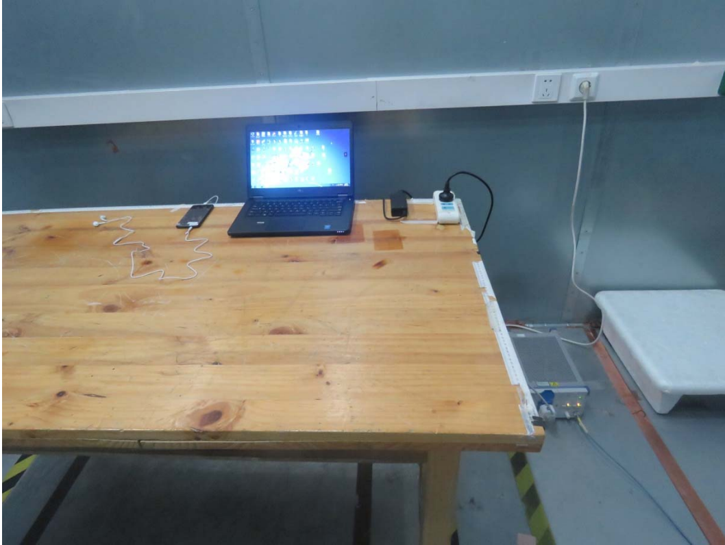
Picture 2 Conducted Emission Test Setup
