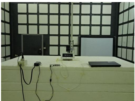
Radiated Emission Set up Photos (Above 1GHz)
