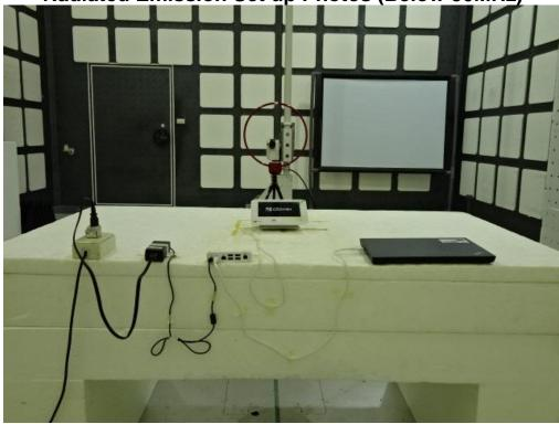
Radiated Emission Set up Photos (Below 1GHz)
