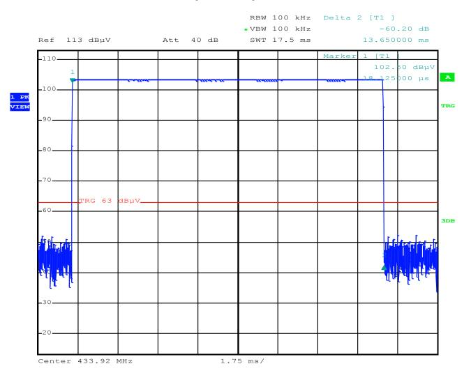
⇒ \* max. Tx on time within a 100 ms time period is 13.65 ms (Marker 1 and Delta 2)
