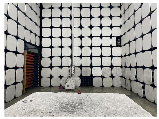
1.1 Set-up for Spurious Emissions below 1GHz
