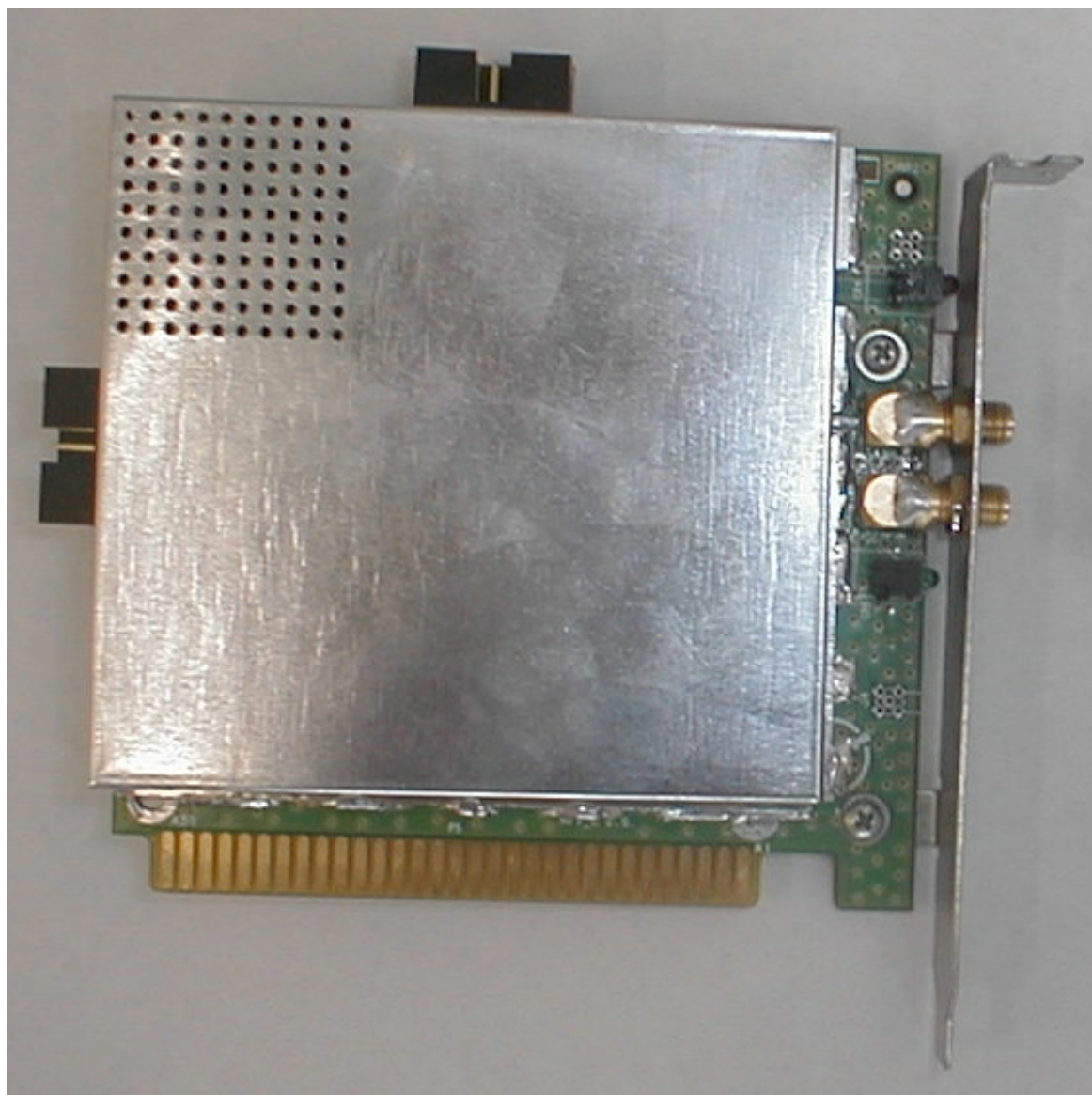
RFU component side with RF shield
