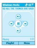
As shown in the figure above, the amount of time elapsed during playback is displayed. In this screen, you can press the Up navigational button to increase volume, or press Down to decrease volume. Press the Right navigational button to start playing the next seguential file, or press Left to play the previous file. Press the Action button to Pause or Play.
