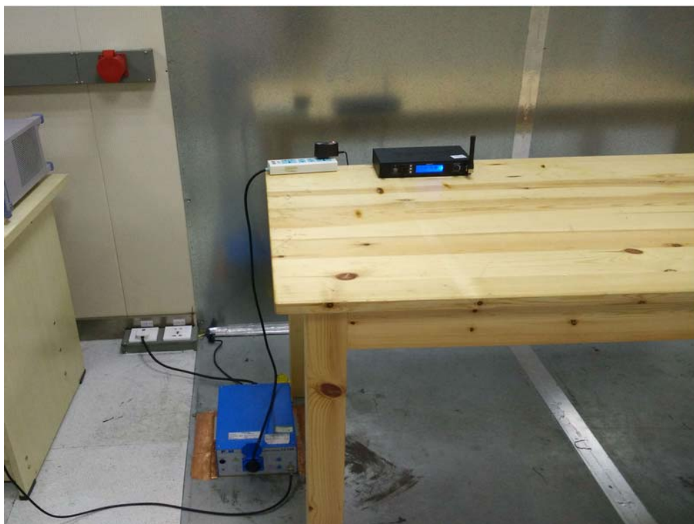
RADIATED EMISSION TEST SETUP
