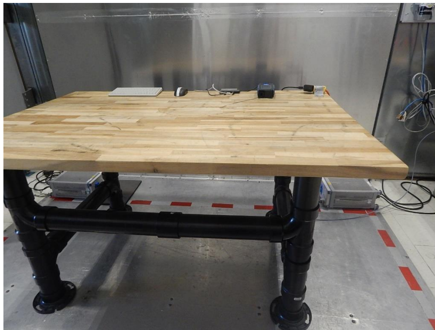
Figure 1.3-1: Conducted emissions – from AC mains power ports setup photo
