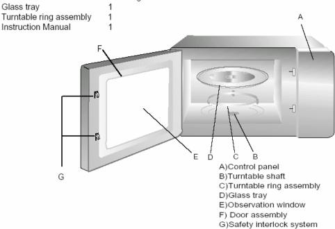
Shuts off oven power if door is opened during operation.
