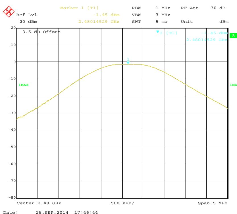
**EDR( $\pi/4$ -DQPSK): Low Channel**
