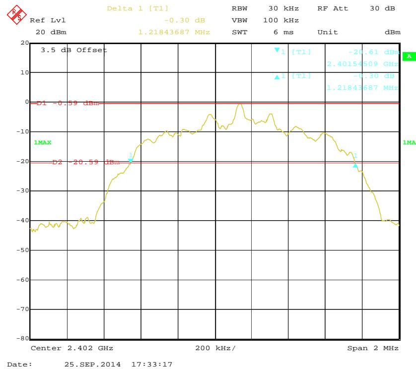
**EDR (8DPSK): Middle Channel**
