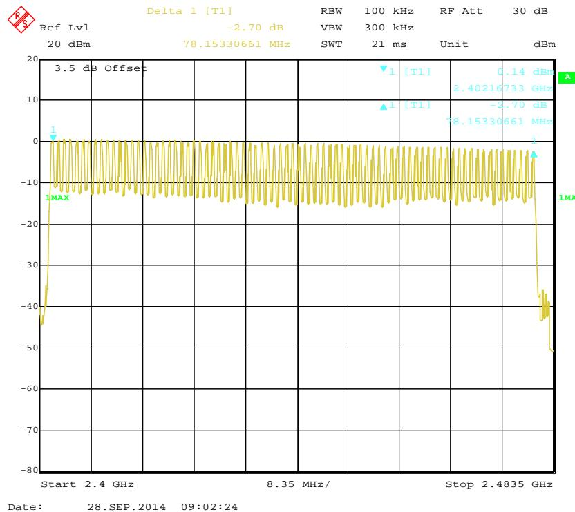
**EDR ( $\pi/4$ -DQPSK): Number of Hopping Channels**
