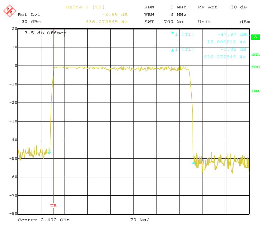
**Pulse time, Middle Channel, 2DH1**
