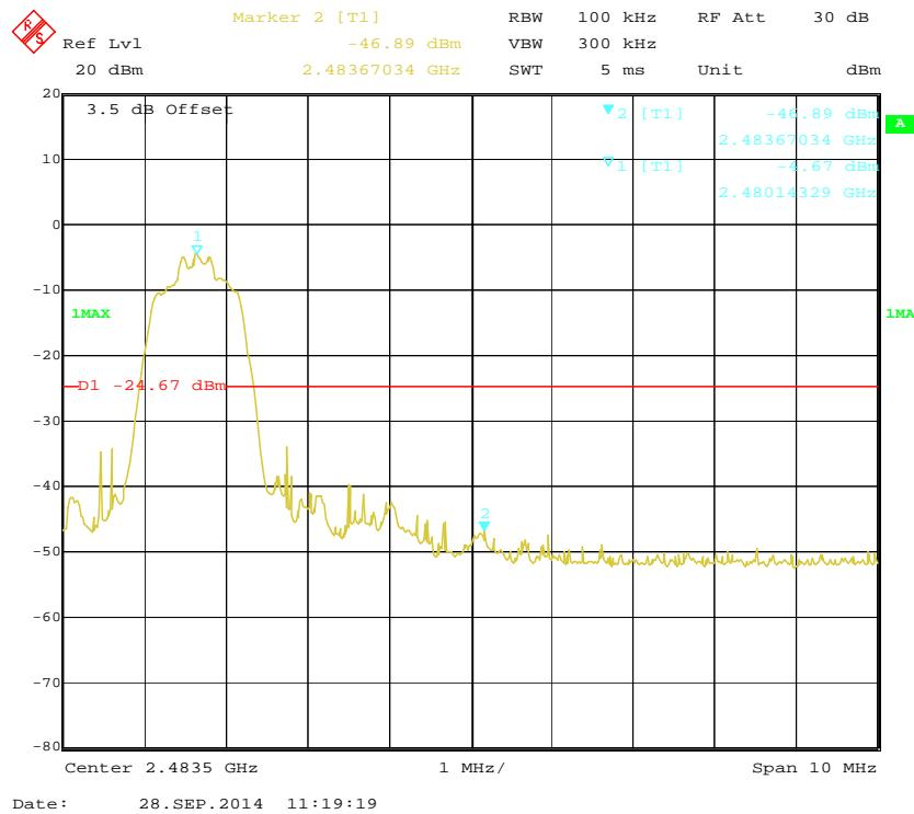
**EDR (8DPSK): Band Edge-Left Side**
