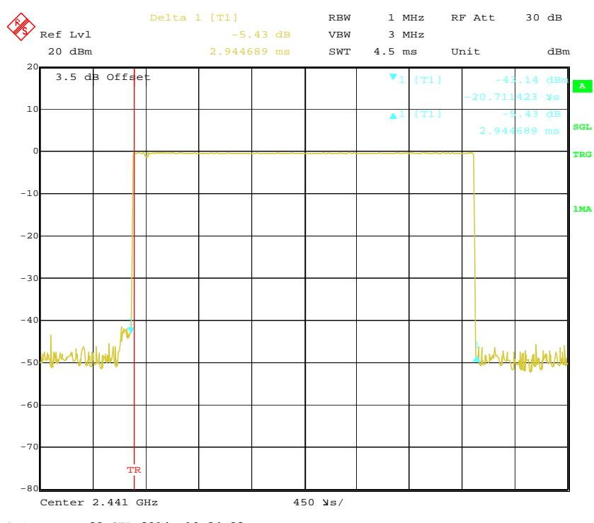
**Pulse time, High Channel, DH5**
