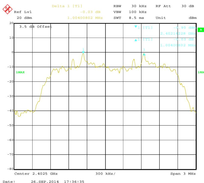
**EDR ( $\pi/4$ -DQPSK): Middle Channel**
