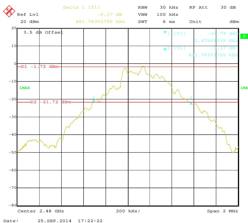
**EDR ( $\pi/4$ -DQPSK): Low Channel**
