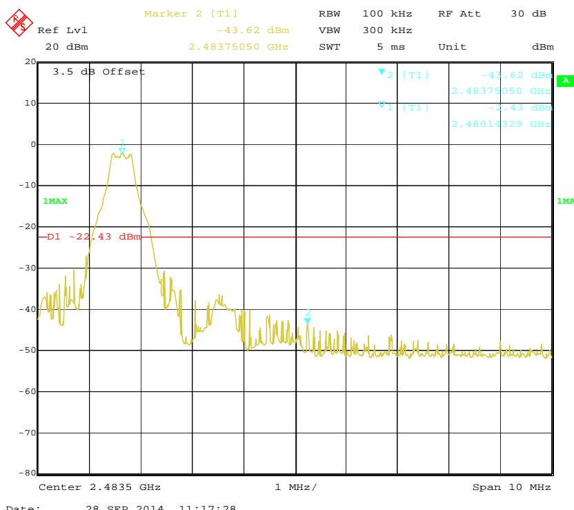
**EDR ( $\pi/4$ -DQPSK): Band Edge-Left Side**
