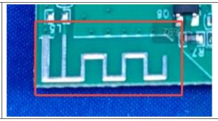
The antenna is PCB antenna.
