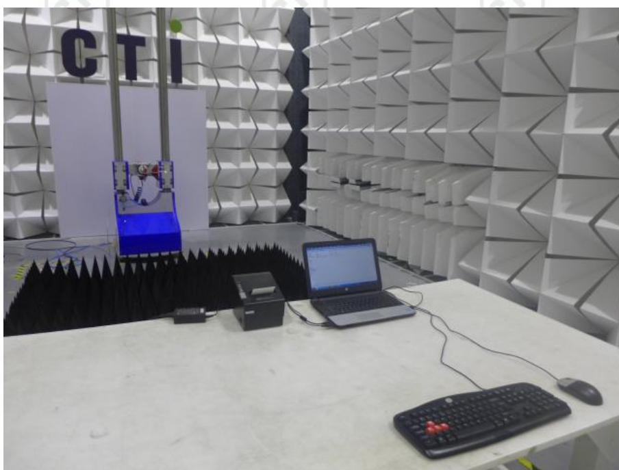
Radiated emission Test Setup (Above 1GHz)
