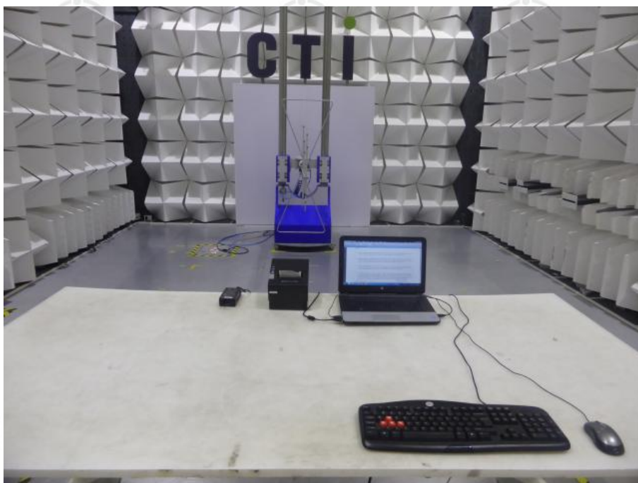
Radiated emission Test Setup (Below 1GHz)
