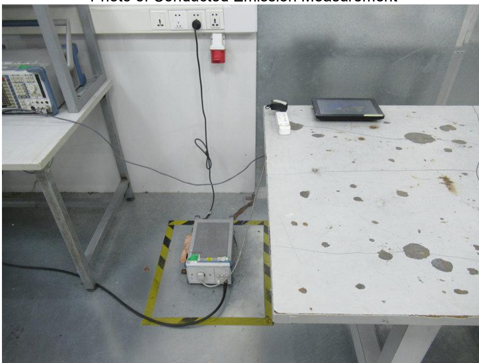
FCC ID: 2AYRW-AT001 Photo of Conducted Emission Measurement
