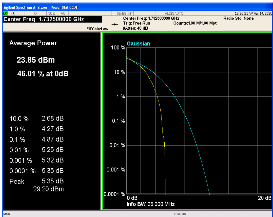
LTE Band4 QAM16 BW=10MHz Channel=20175 RB Size=1 Position=#0
