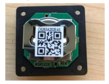
**Step #2:** Remove the lid with attached pcb from the case.
