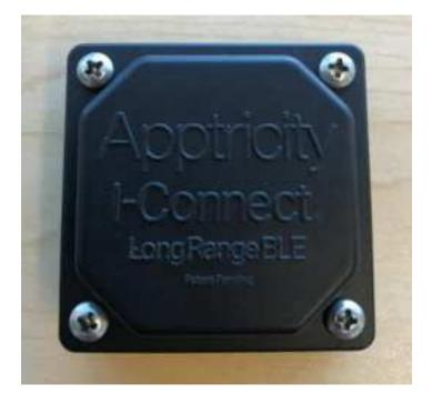
**Step #1:** Remove the 4 screws from the top of the case.
