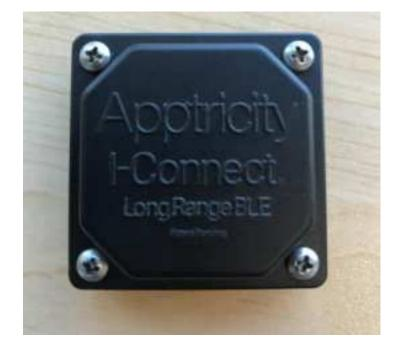
**Step #6:** Replace the four screws to attach the top to the bottom of the case.
