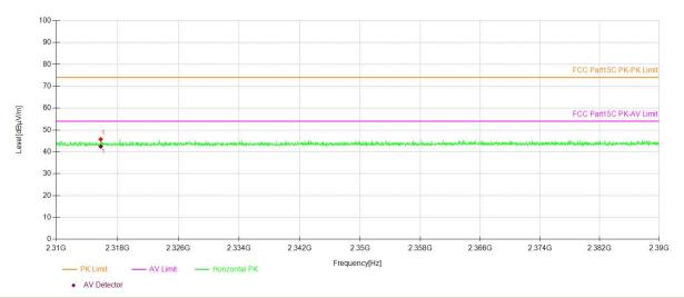
Test Model Spurious Emission in Restricted Band2310-2390MHz
