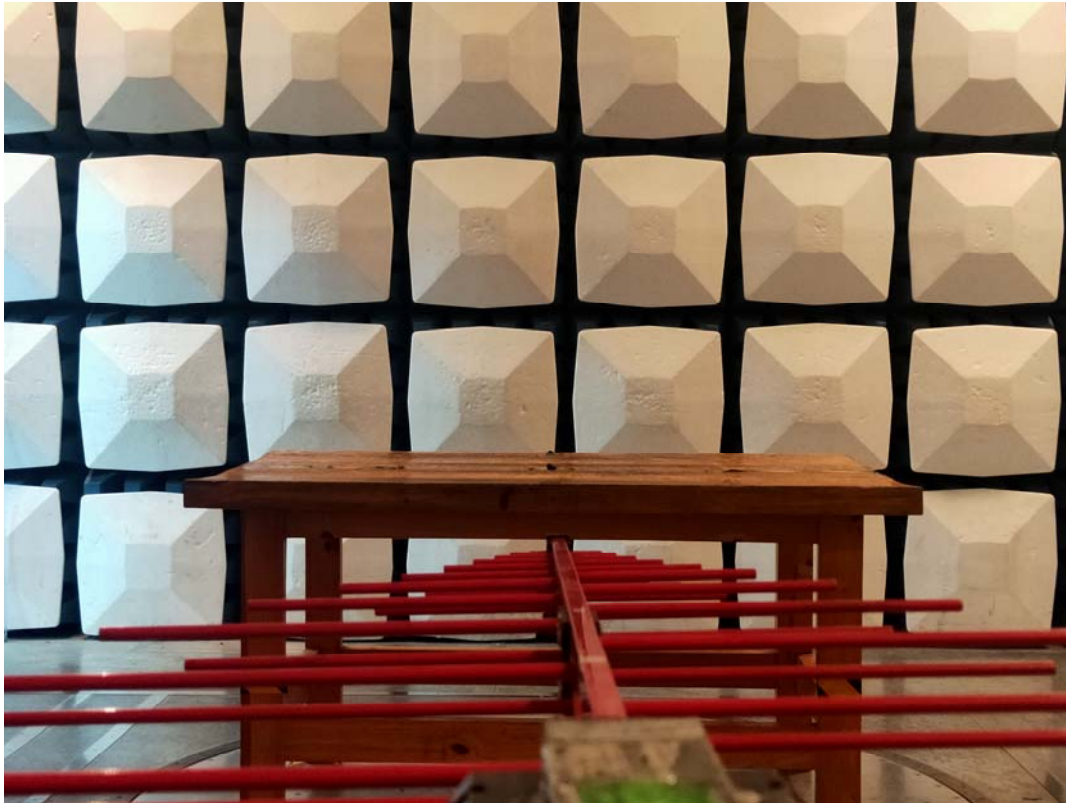
Radiated Emission Above 1GHz View
