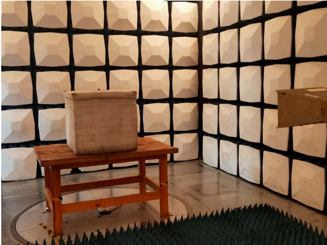
Radiated Emission Above 1GHz View
