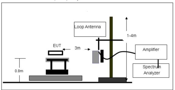
(B) Radiated Emission Test-Up Frequency 30MHz~1GHz
