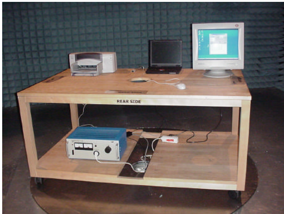
Picture 1 : Setup for radiated emission tests below 1 GHz
