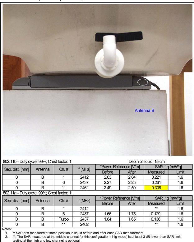
3. Spacing between host device and phantom: 0 mm
