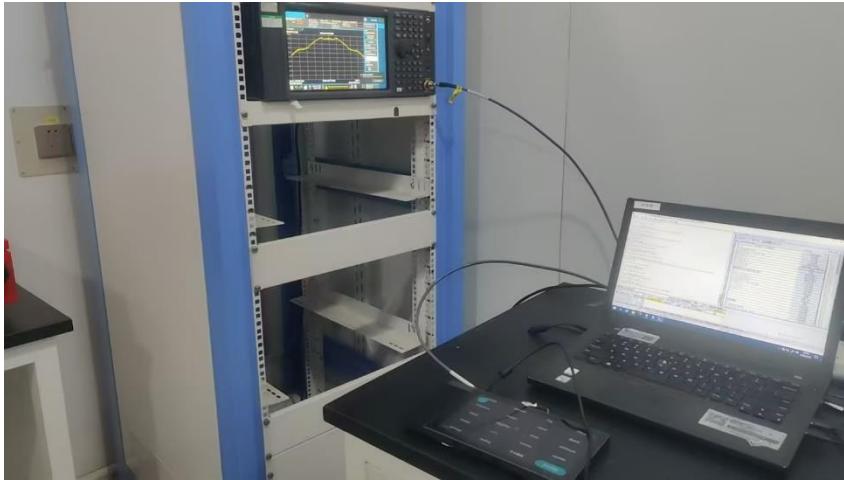
RF Conducted setup
