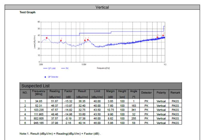
2. Factor (dB) = Antenna Factor (dB/m) + Cable loss (dB) - Pre Amplifier gain (dB).
