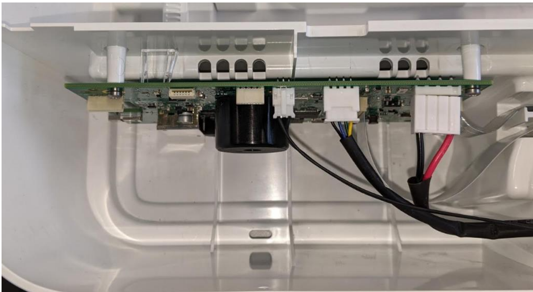
Figure 3: Control board as mounted in unit.
