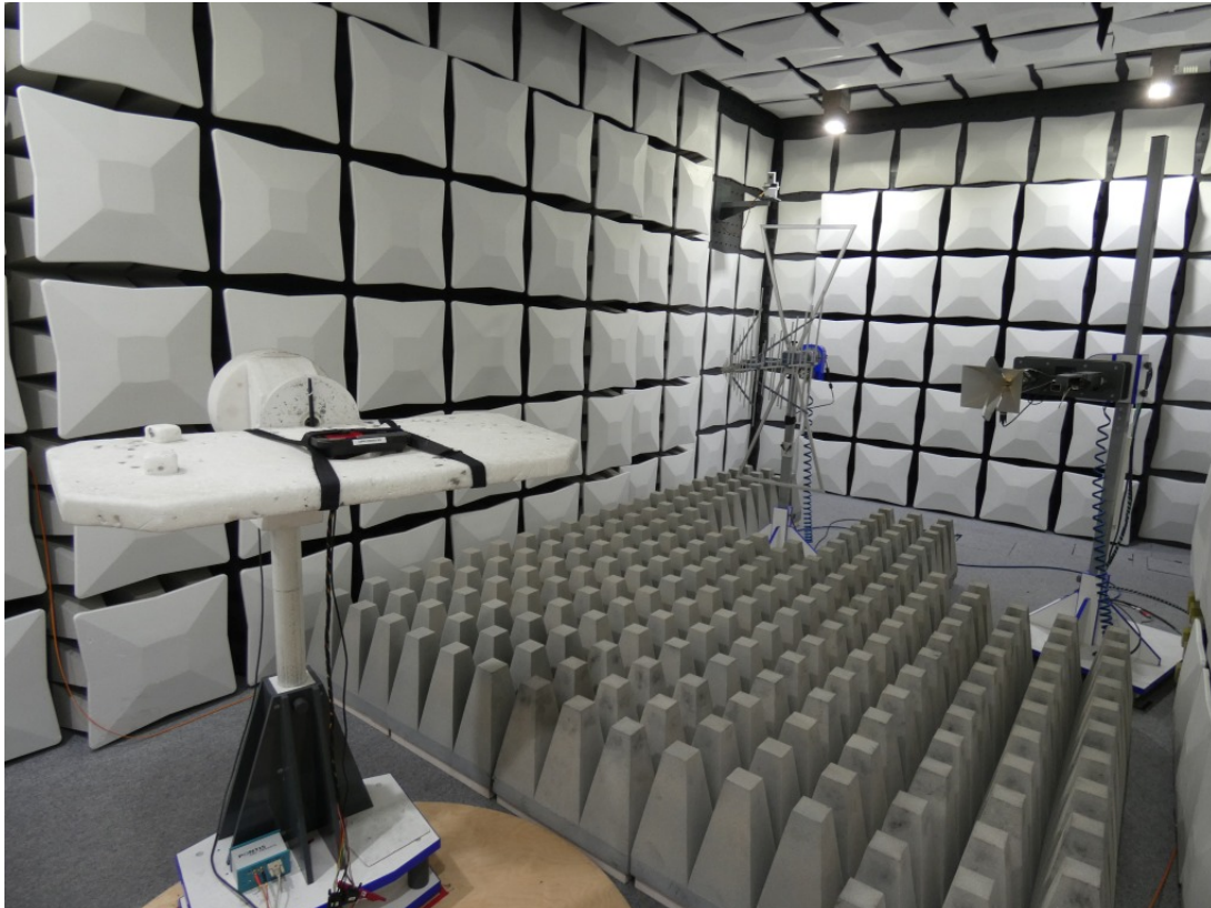
Photo 8: Setup for radiated emissions > 1 GHz, total view
