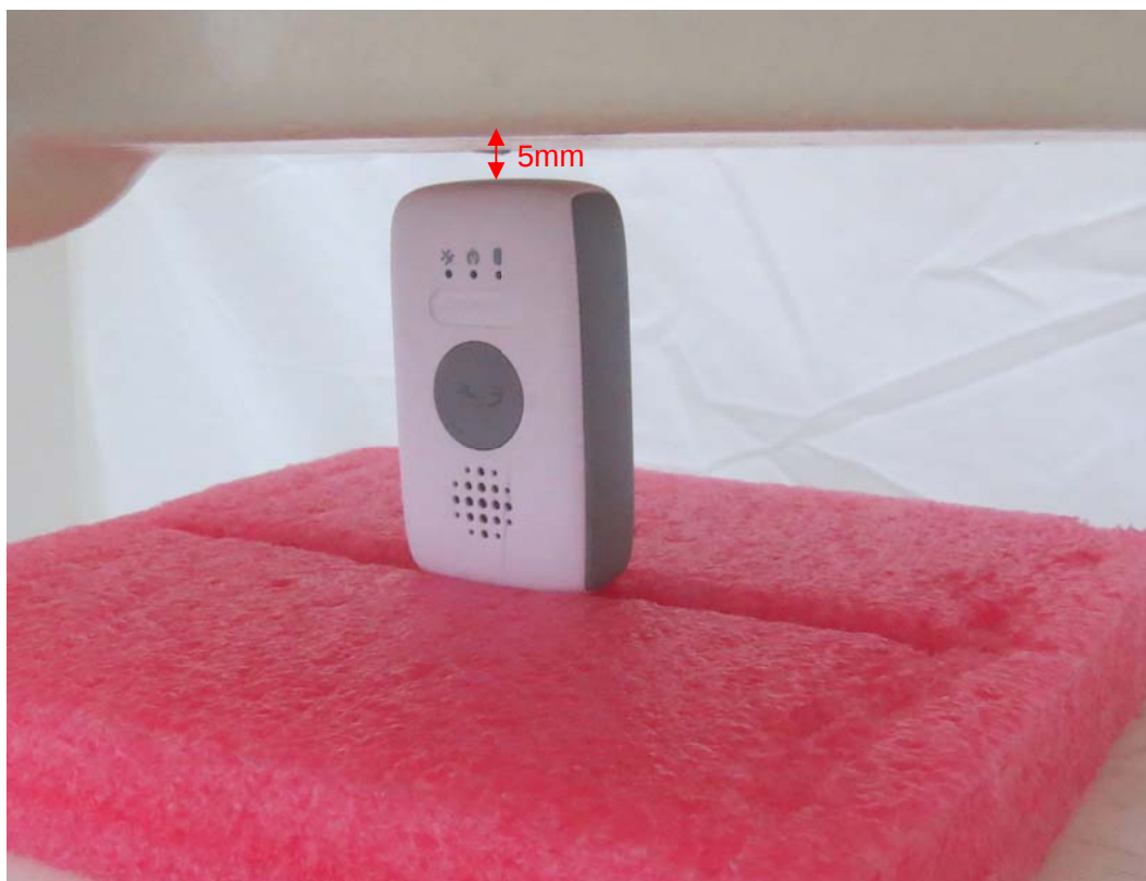
Picture 5: Bottom Side, the distance from handset to the bottom of the Phantom is 5mm
