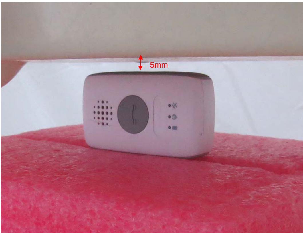
Picture 4: Right Side, the distance from handset to the bottom of the Phantom is 5mm
