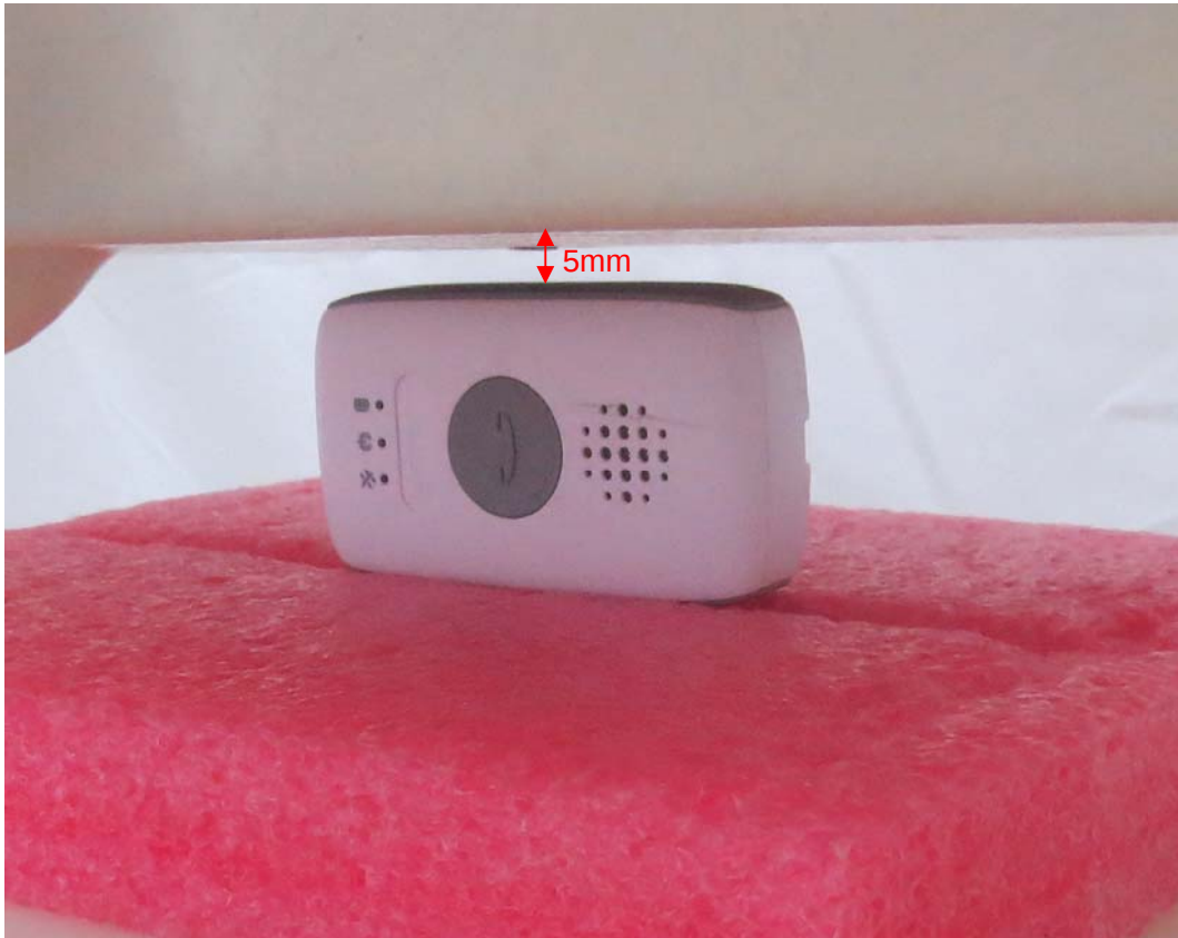
Picture 3: Left Side, the distance from handset to the bottom of the Phantom is 5mm
