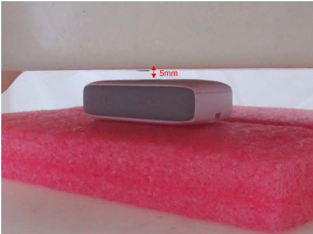
Picture 2: Front Side, the distance from handset to the bottom of the Phantom is 5mm
