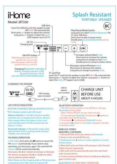
Long press and hold + and - button for 3 seconds to reset.
