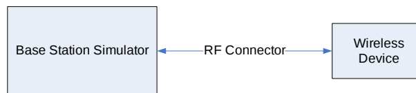
Figure 8-2 Power Measurement Setup
