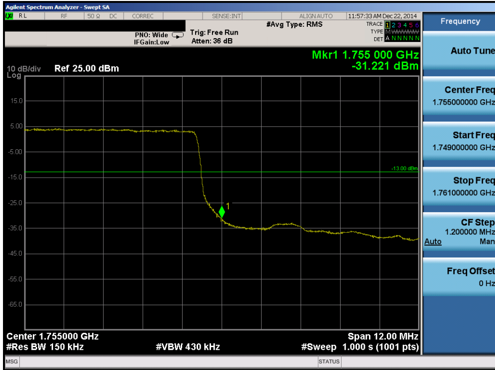
Plot 6-29. Upper Band Edge Plot (Band 4 – 15.0MHz QPSK – RB Size 75)
