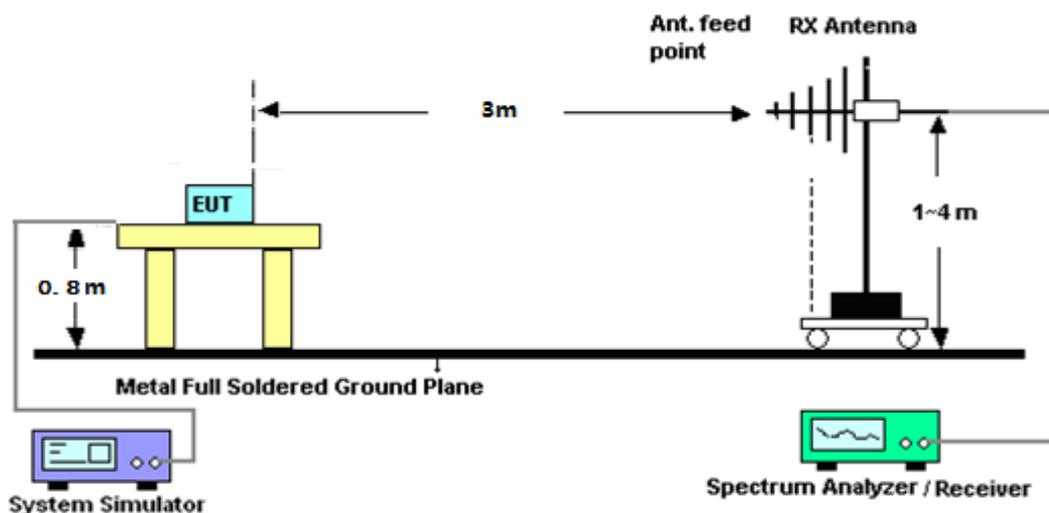
For radiated test from above 1GHz
