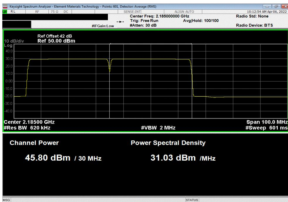
AWS Multicarrier Multiband, Port 1, Test Case 3: AWS Band NR30 (2 Carriers), PCS Band NR30 (Single Carrier), 256-QAM Modulation, PCS Single Carrier, 1962.5 MHz..
