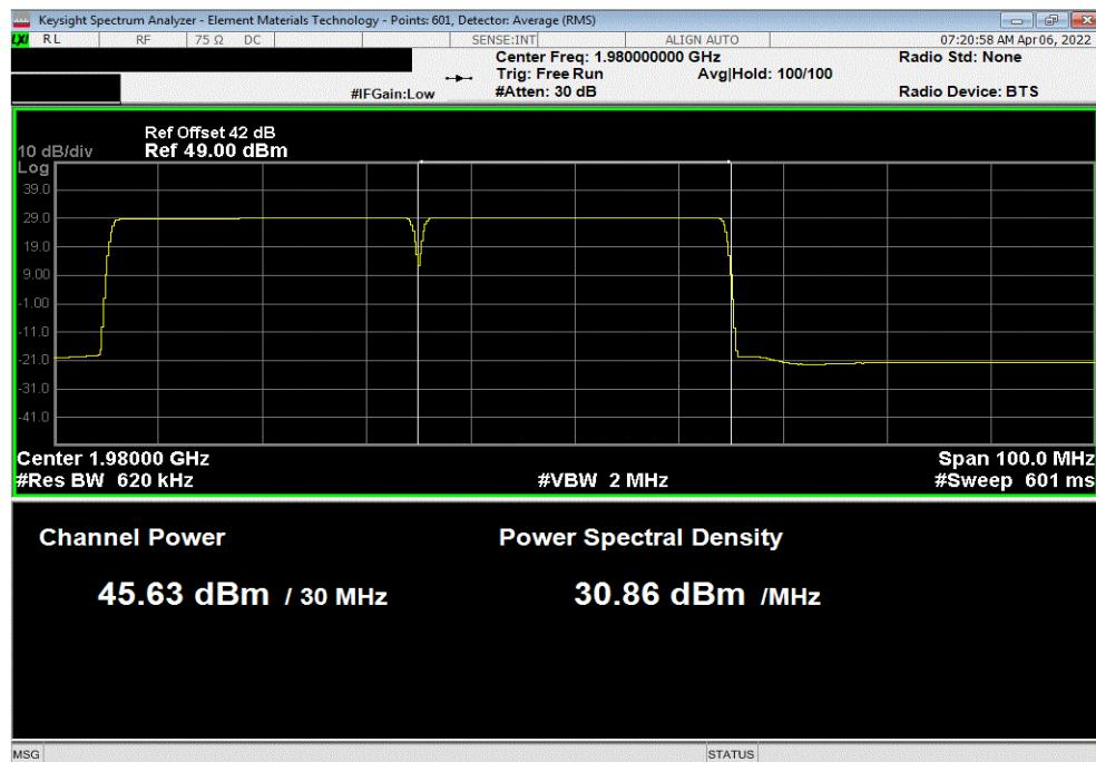
PCS Multicarrier Multiband, Port 1, Test Case 3: PCS Band NR30 (2 Carriers), AWS Band NR30 (Single Carrier), 256-QAM Modulation, AWS Single Carrier, 2155 MHz..
