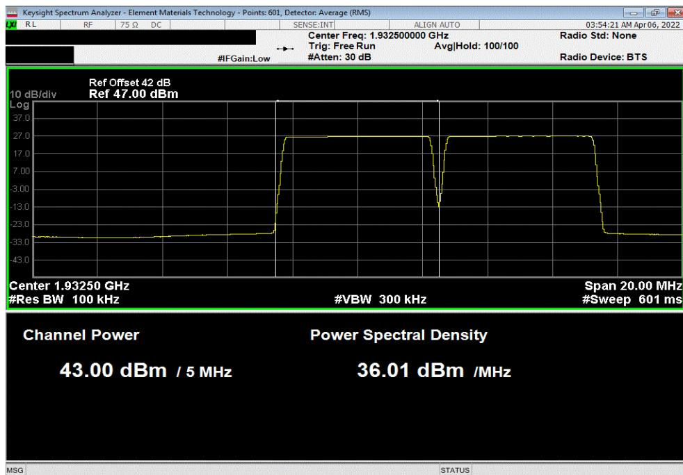
PCS Multicarrier Multiband, Port 1, Test Case 1: PCS Band NR5 (3 Carriers), AWS Band NR5 (Single Carrier), 256-QAM Modulation, PCS Carrier 2, 1937.5 MHz
