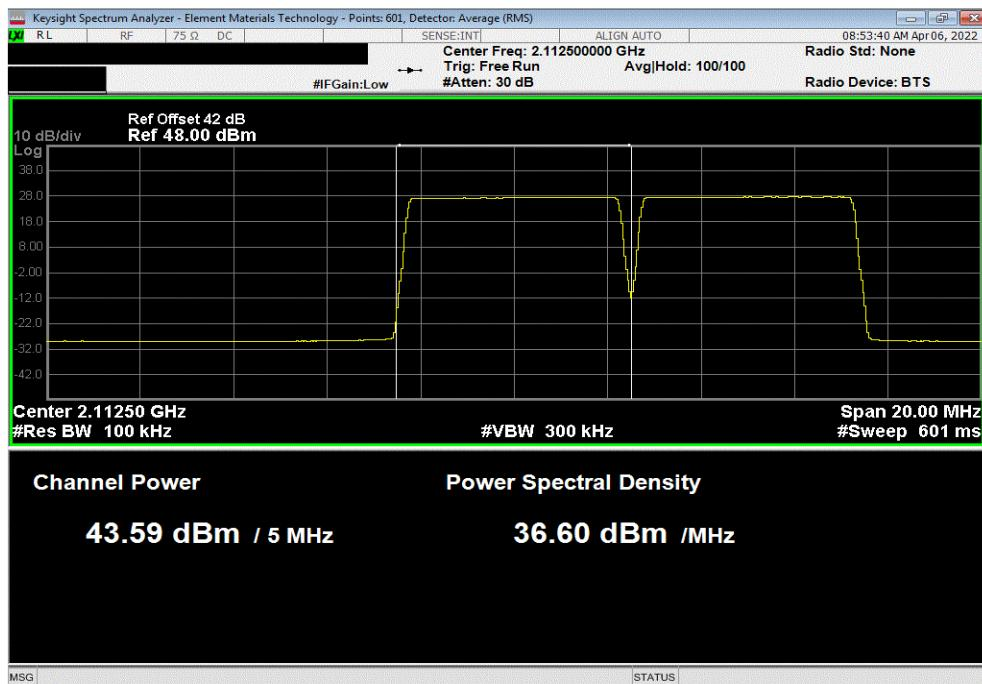
AWS Multicarrier Multiband, Port 1, Test Case 1: AWS Band NR5 (3 Carriers), PCS Band NR5 (Single Carrier), 256-QAM Modulation, AWS Carrier 2, 2117.5 MHz
