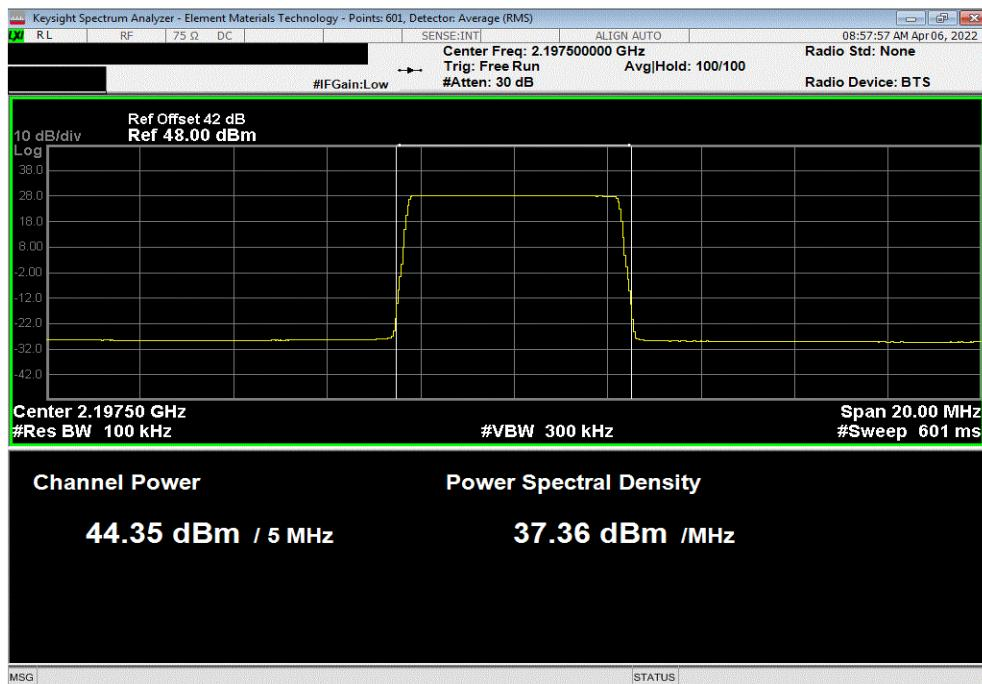
AWS Multicarrier Multiband, Port 1, Test Case 1: AWS Band NR5 (3 Carriers), PCS Band NR5 (Single Carrier), 256-QAM Modulation, PCS Single Carrier, 1962.5 MHz
