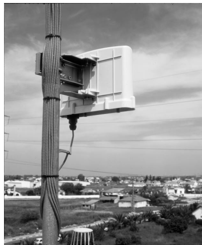
Figure 8-3: Typical SPR mounted outdoors on a pole
