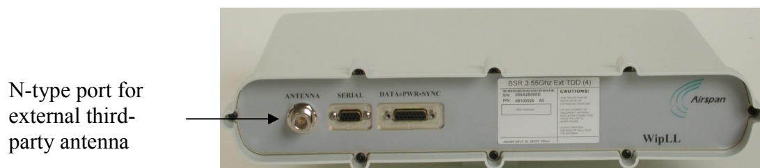
Figure 7-4: BSR model with one N-type connector
