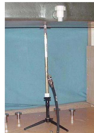
2450MHz Dipole Setup (Planar Phantom)
