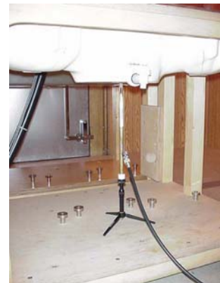
2450MHz Dipole Setup (SAM Phantom)
