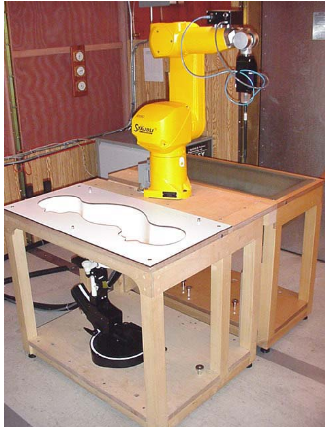
DASY4 SAR Measurement System with SAM phantom
