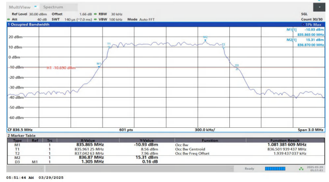
Band26(824-849)-1.4MHz-16QAM-26915-6RB#0-PASS
