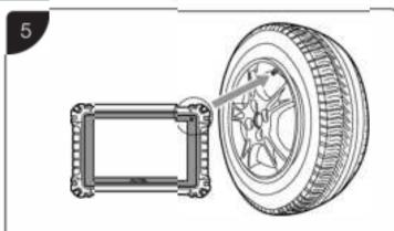
Hold the MaxiSys MS906 Pro-TS tablet with its top right corner close to the tire sidewall at the valve stem to activate the TPMS sensor.
