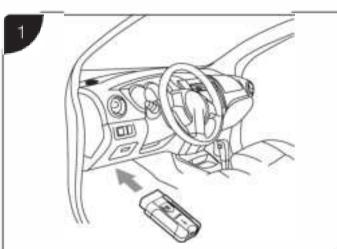
Insert the Vehicle Data Connector on the MaxiVCI V200 into the vehicle's DLC, which is generally located under the vehicle dashboard.
