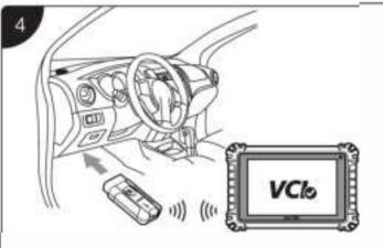
When the MaxiVCI V200 is properly connected to the vehicle and the tablet, the VCI status button on the bottom bar of the screen will display a green badge with a check mark at the corner indicating the tablet is ready to start vehicle diagnosis.
