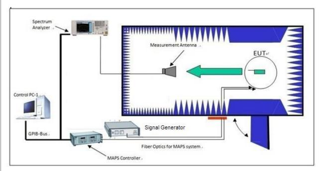
Figure 1. 2D antenna pattern test system.
