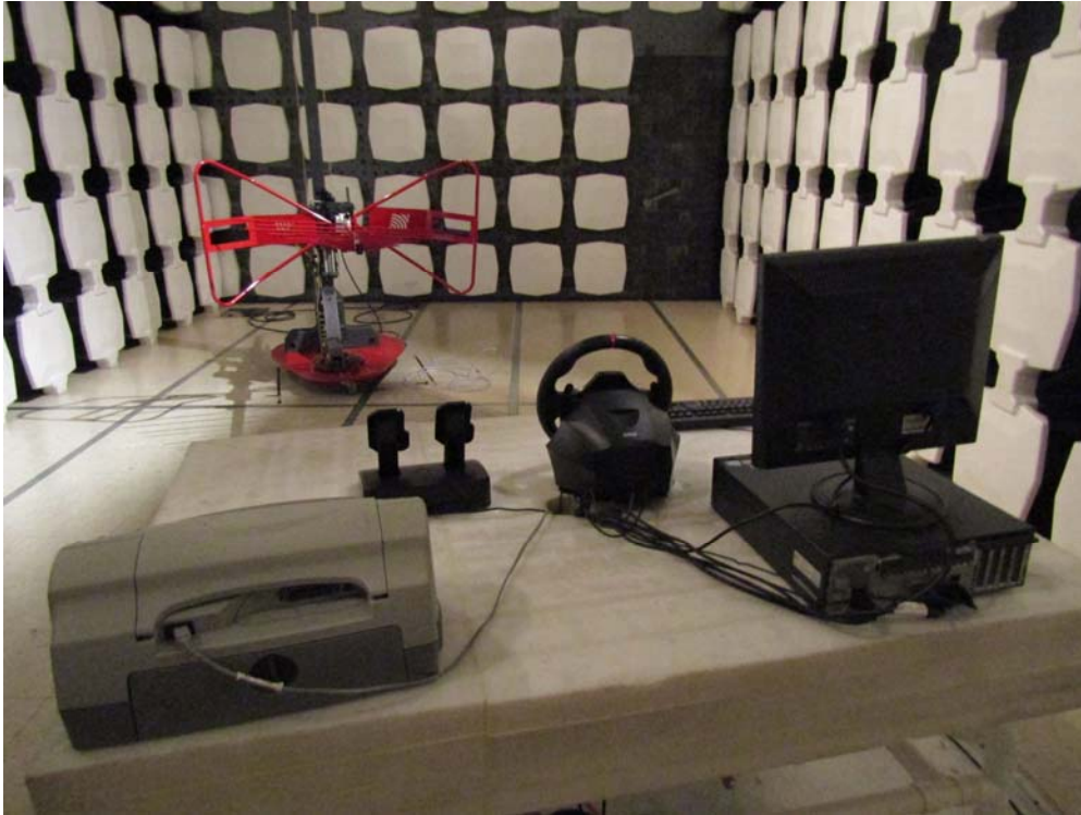
Measurement of Radiated Emission Test Set Up
